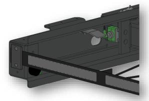
It is possible to place a sensor to detect a folded bumper
